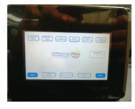
All the data that appear on the operator panel can be extrapolated from the PLC remotely through the Link: IP 10.VPNIN-STANCE: \*\*\*\*\* / (serial number) .HTM this is possible thanks to a RUT240 4G modem router (photo 4) which with a special dedicated SIM allows both the connection and the display of data and information necessary for both remote assistance and software modification.
