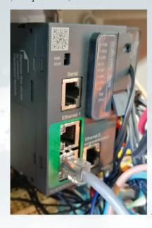
This **PLC** is able to provide a multiplicity of information that can be displayed on the latest generation control panel mod. MAGELIS SCHNEIDER 7.5 "LCD touch screen, (see photo 2)
