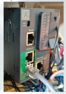
This **PLC** is able to provide a multiplicity of information that can be displayed on the latest generation control panel mod. **MAGELIS SCHNEIDER** 7.5 "LCD touch screen, (see photo 2)
