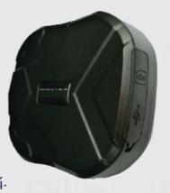
The latest generation magnetic **GPS** Tracker *(photo4)* allows not only to know where the vehicle is but also to have a track of the route it has traveled with excellent precision.
